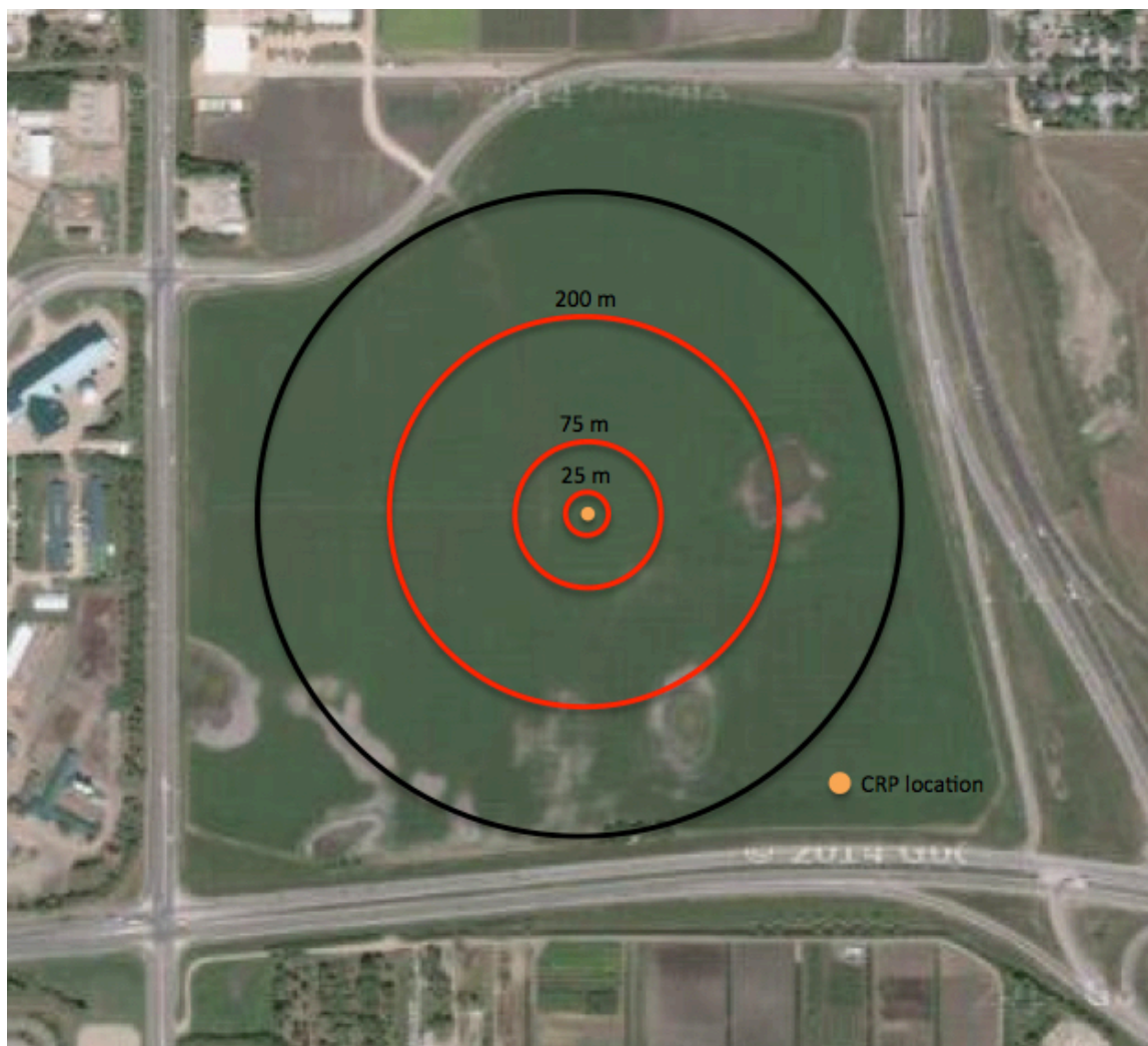
Figure 4.1. Location of CRP and estimated 300 m radius measurement footprint (black radial). The red lines represent the sampling radials. Image from Google Maps.
