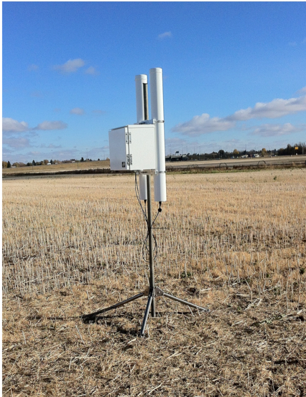
Figure 2.1. Image of the Cosmic-ray soil moisture probe (CRP) installed in an agriculture field.
