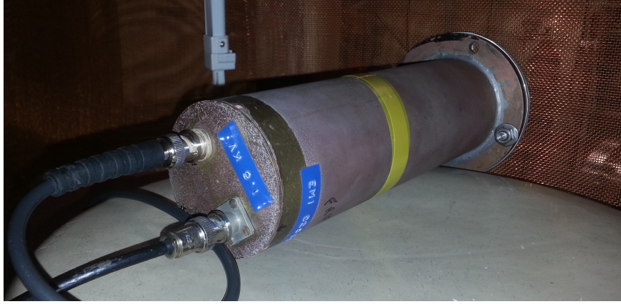
Figure 4.18: Picture of the assembled scintillated PMT for detecting hard x-rays situated 2 meters away from the chamber in the Faraday cage, directly facing the anode tip.
