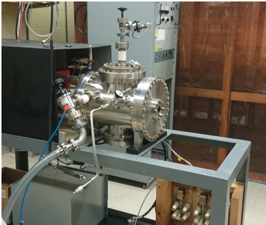
Figure 4.1: The UofS-I dense plasma focus device. A control panel is situated beside the DPF device, and a Faraday cage built by means of copper mesh encloses the signals measurement devices.
