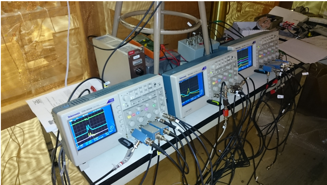
Figure 4.21: Tektronix oscilloscopes (TDS 2024c) for signals measurement and recording, with attached USB flash drives for storage. Each oscilloscope inputs 4 channels triggered by a common signal.
