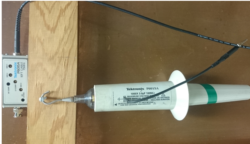
Figure 4.12: A Tektroniks P6015a voltage probe used to measure the voltage of the DPF anode.
