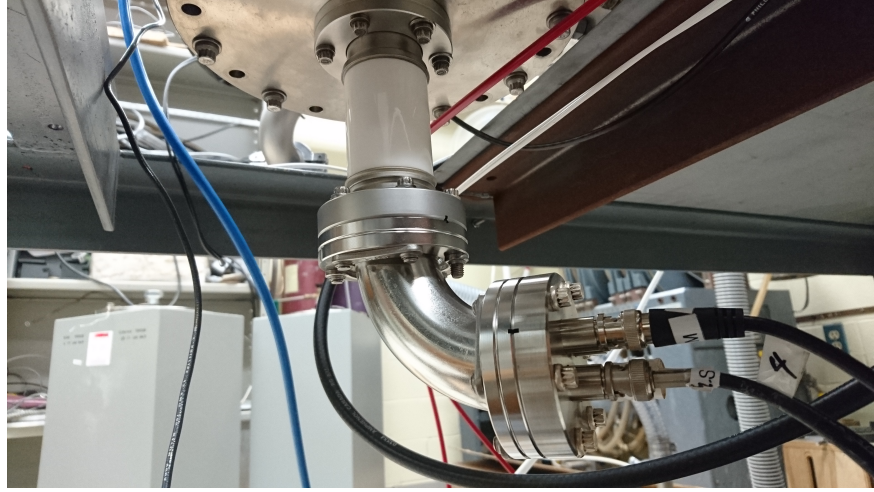
Figure 4.16: A 4-PIN photodiode array attachment under the chamber to allow more simultaneous detection of SXR per shot.
