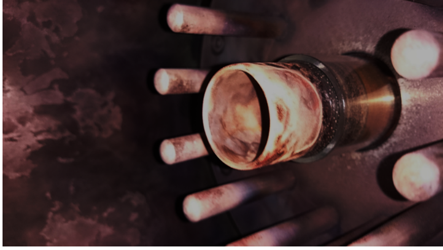
Figure 4.2: Electrodes in vacuum: a hollow copper anode nested in 12 concentric cathode rods, and a quartz-infused glass insulator separating the electrodes.
