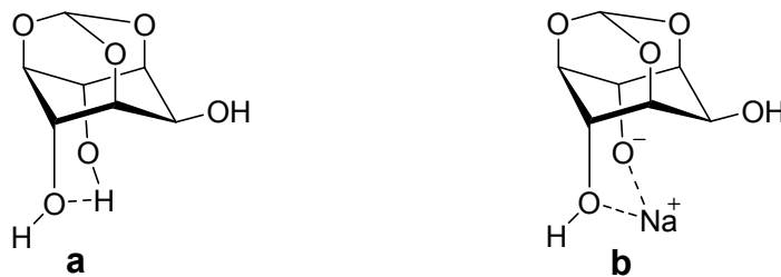
Figure 12. Rationalization of the regioselectivity demonstrated by the orthoformate of myo -inositol: a illustrates the intermolecular hydrogen bond accounting for the lower pKa at the C-4 and C-6 hydroxyl groups; b illustrates the chelate formed upon reaction of the orthoformate with a metal hydride
