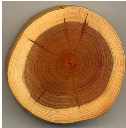
Fig. 2.1 Yew wood ( Taxus baccata ) where the lighter part is sapwood and the darker part is heartwood. (Original source: Photo: MPF, November 2004, GNU Free Documentation License)
