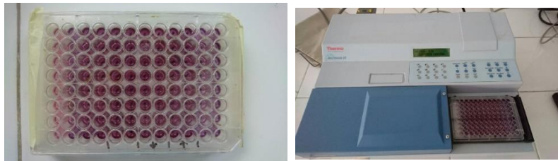
Figure 1. Cytotoxicity test on 96 well plates that was monitored by ELISA reader
