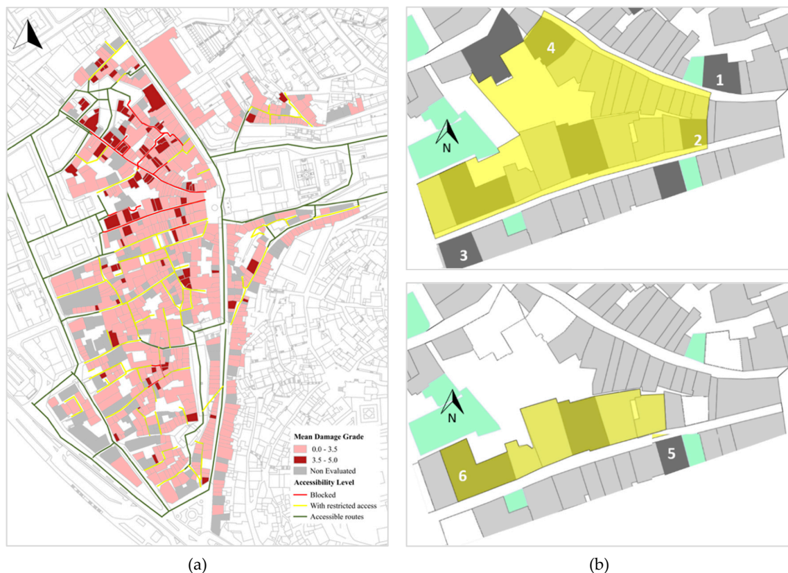
Figure 4. Mapping of (a) evacuation routes and (b) configuration of the most critical urban area before (top) and after (bottom) retrofit, adapted from Aguado et al. [31].
