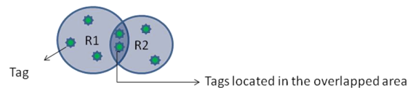
Figure 7. Tags Located in the Overlapped Area
