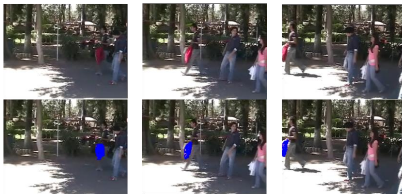
Figure 4.10. Image sequence as processed by the LVQ segmentator while segmenting for the backpack within an outdoor environment.
