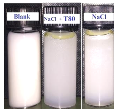
Figure 1. Influence of different diluted solutions on the stability of 2.5% oregano essential oil nanoemulsions: 1:1 (v/v) dilution in distilled water (blank) was compared to 3.4 M NaCl and 0.5% T80 and 3.4 M NaCl (pictures after 1 h at 20^\circ\text{C} ).
