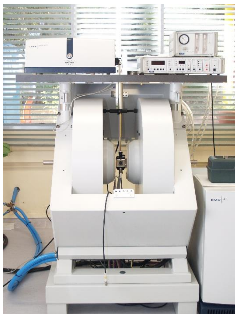
Fig. 35. Bruker EMX spectrometer from IQAC-CSIC facilities. [34]
