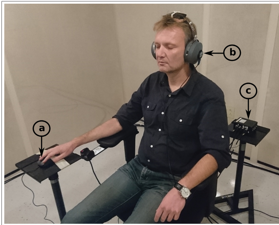
Figure 2.1 (Color online) Subject wearing the HPs (b) and adjusting the mouse wheel (a) used for loudness equalization in the audiometric sound booth. The earpieces are fitted onto the subject's ears, under the HPs, and the microphones are connected to the battery-powered signal conditioning box (c) behind the subject
