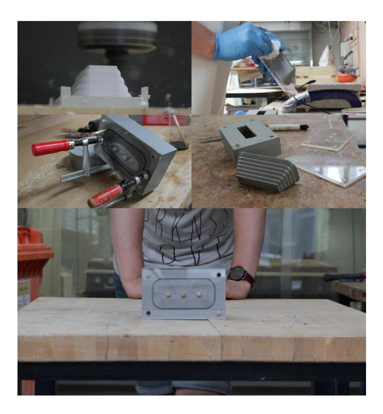
expense. In order to cut costs, excess material was removed from around the mould. In order to see the flow of silicone through the mould it was printed in a semi-clear material. The idea was to cast multiple pieces using silicone with different hardness's. This would be done by adding silicone oil to the two-part silicone mix in a controlled and documented manner. However, the first cast proved that the mould could not withstand the pressure of de-moulding and it was broken entirely.
