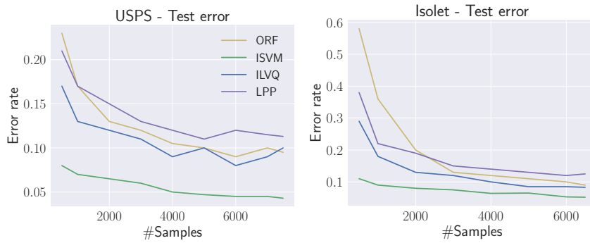
Figure 3.15: Learning curves of tree - and instance based models in comparison. Instance based methods are particularly at the beginning more accurate and with a steeper learning curve.
