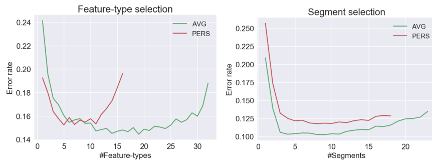
Figure 5.13: Forward feature selection in two steps: First, the best feature types are determined using all segments (top). Subsequently, the most valuable segments are determined on the basis of the three best feature types (bottom). The personalized model had no access to the normalized features because they have no effect on its performance. The number of evaluated segments depends on the chosen feature types in the first step. Hence, the number of evaluated segments is different for both models.
