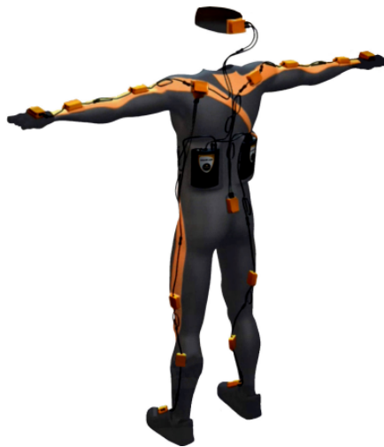
Figure 5.10: The Xsens body suit with 17 IMU sensors. The sternum IMU is occluded due to the image perspective. We used the wireless version. Source: https://www.xsens.com/ .
