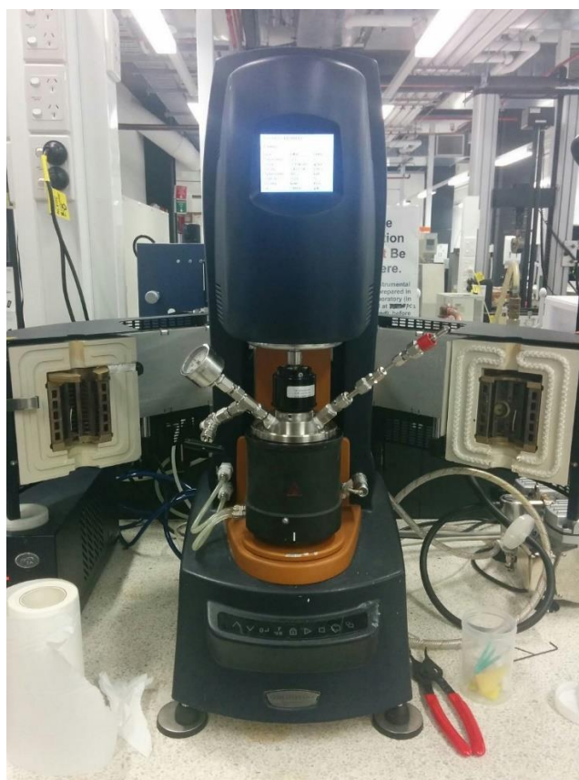
Figure 3. 8 – Rheometer (HR3, TA Instruments) with pressure cell attached for measuring sludge at high temperature and high-pressure conditions.
