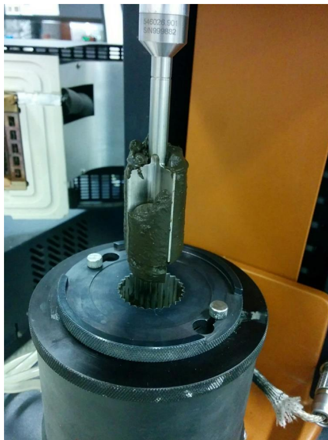
Figure 3. 17 – Viscoelastic measurement of 12 wt% waste activated sludge using vane geometry, showing the thickened sludge did not shear properly due to formation of gap between the rotor and the shearing surface of the cup.
