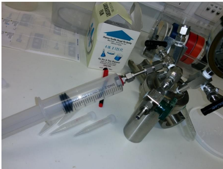
Figure 3. 7 – Modified syringe connected to sample inlet valve of pressure vessel to allow sludge to be loaded into reactor from the bottom of the vessel.
