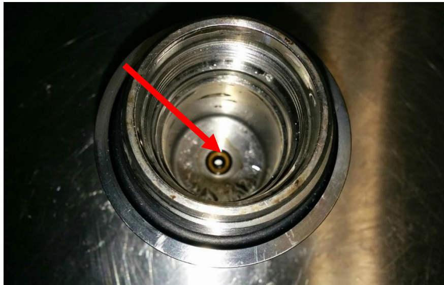
Figure 3. 11 – Pressure cell bearing exhibiting signs of condensation, suspected to increase bearing friction and affect measurement results.
