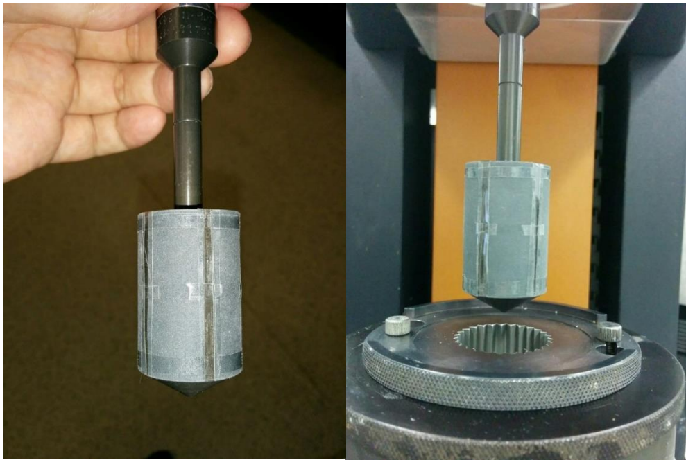
Figure 3. 15 – Concentric cylinder rotor with sandpaper attached to the shearing surface to reduce slippage effects.
