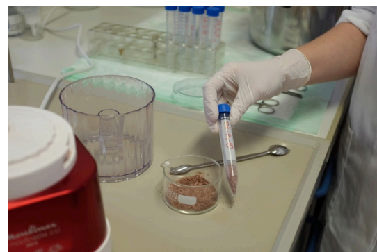
Figure 9: Dehydrated slices of raw placental tissue were ground and samples taken from the powder.
