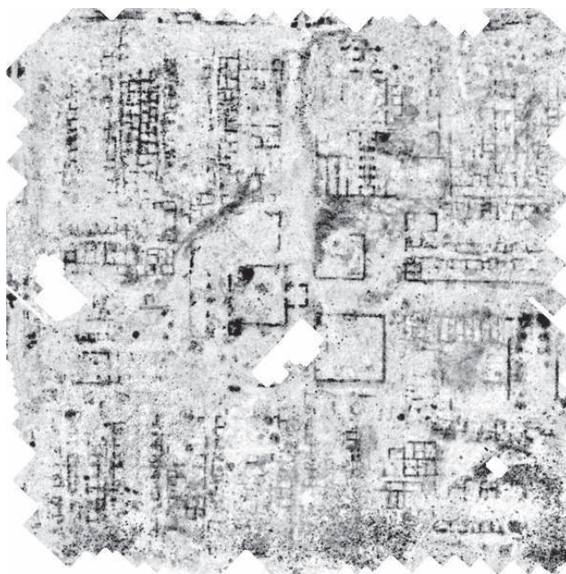
Figure 2: GPR depth slice 0.20-0.40 m. Archaeological structures show partly very good and partly very small contrast and are overlaid by striping patterns in the measuring direction.
