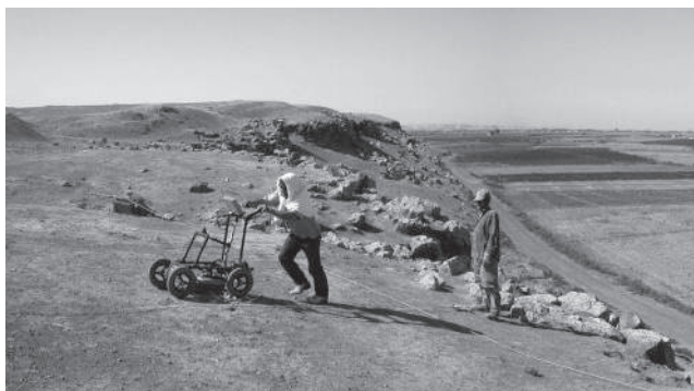
Figure 1: GPR prospection at the edge of the plateau immediately north of the Roman fort of Qreiye using a Sensor&Software Noggin System with 500 MHz antennas.
