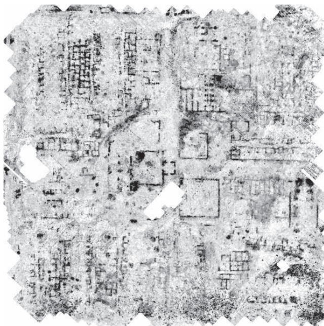
Figure 3: GPR depth slice 0.20-0.40 m. The striping patterns disappear with the use of an average trace removal filter with only 1 m length.
