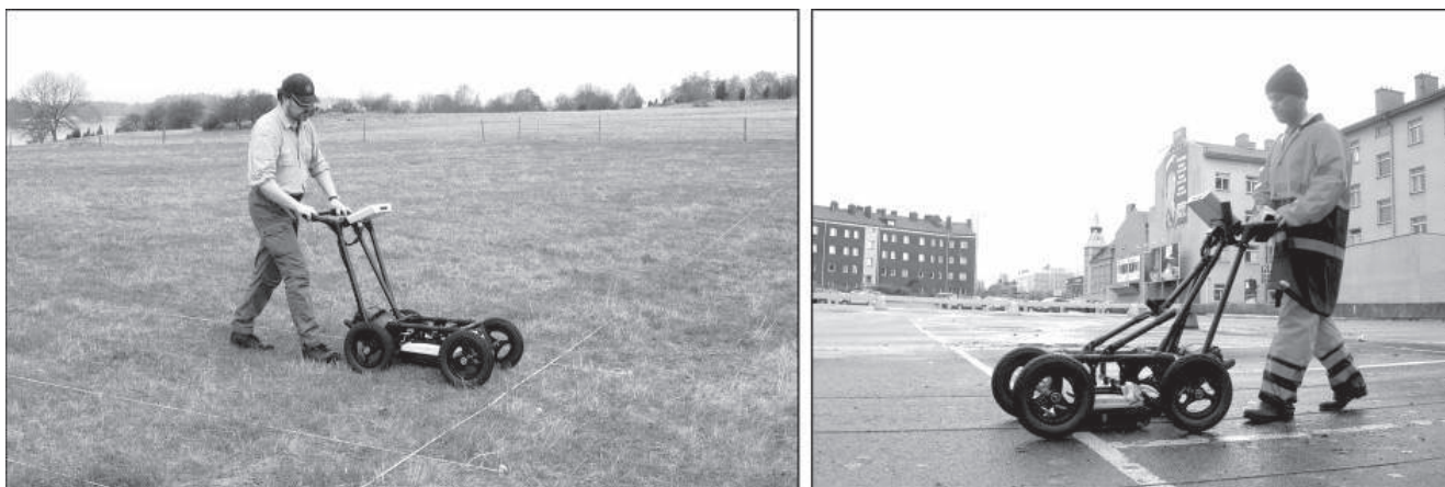
Figure 1: GPR surveys in the urban centre of the Viking town Birka (left) and in the city of Norrköping (right).
