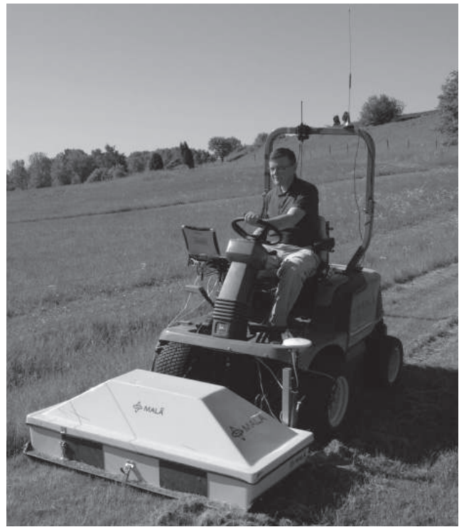
Figure 3: High resolution multi channel GPR survey using the Malå Imaging Radar System MIRA at the Viking age town Birka, Sweden 2008. Photo: Bernth Johansson Malå Geoscience.
