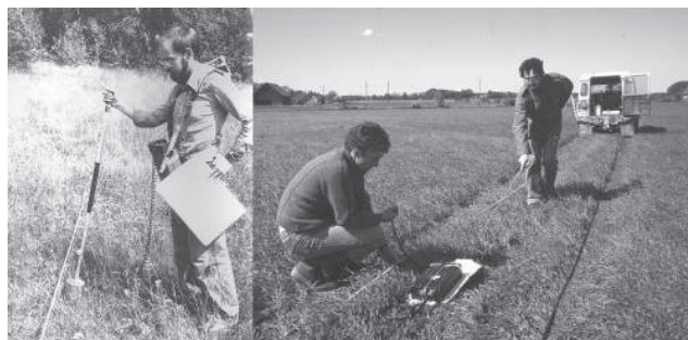
Figure 2: (left) Measurements with a proton-magnetometer at the Stone Age site in Gömme, Sweden. © Swedish National Heritage Board. (right) Early GPR measurements at the Stone Age site Ajvide, Gotland, Sweden. Photo: Göran Burenhult.
