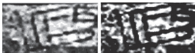
Figure 3: Classified magnetic data (left) and result of the fusion between the classified magnetic image with the denoised resistivity image (right).
