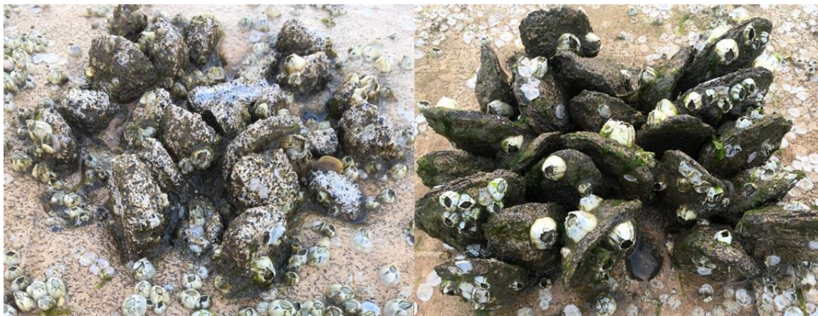
Figure 17. (Left) substrate constructed with magnesium supplement observed greater erosion than the substrate constructed with standard concrete (right).
