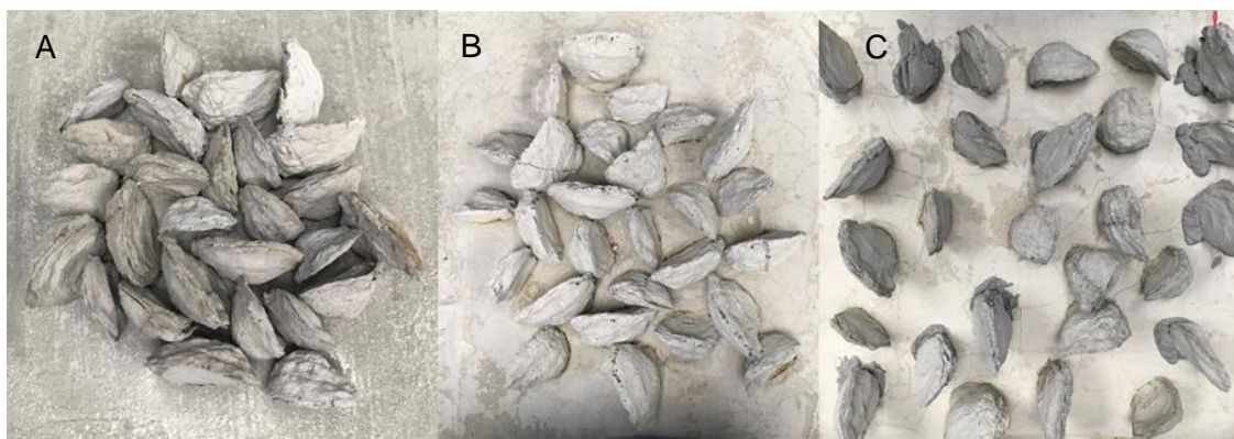
Figure 8. Concrete tiles with artificial shells created with 3 levels of interstitial space: (a) low, (b) intermediate, and (c) high respectively.
