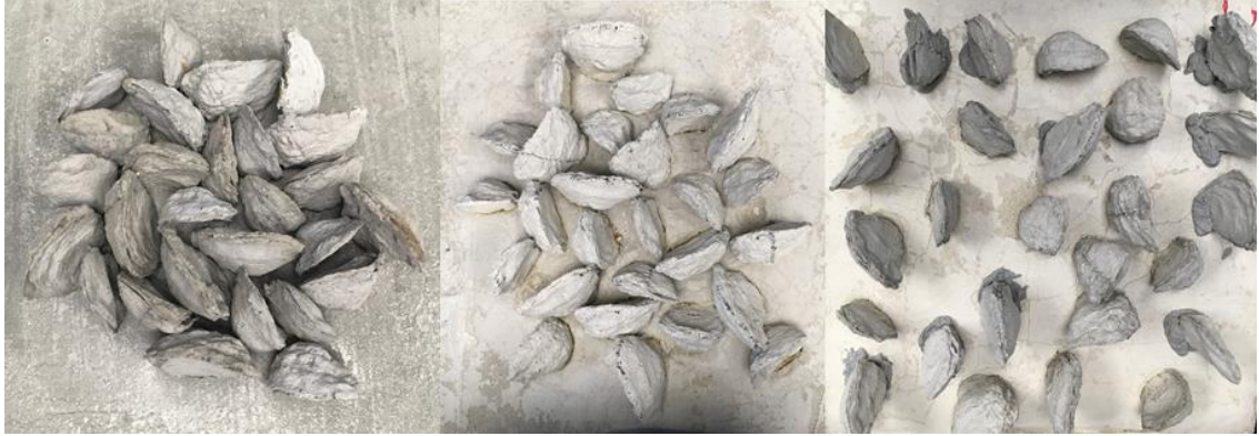
Figure 22. Constructed artificial oyster substrate with low, intermediate, and high interstitial space respectively.
