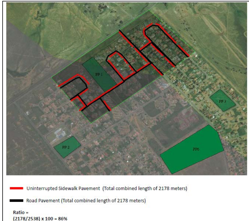
Figure 1: Pedestrian facility network to road network ratio for public parks in a residential area
