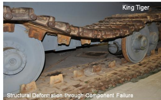
(b) Structural deformation due to component failure
