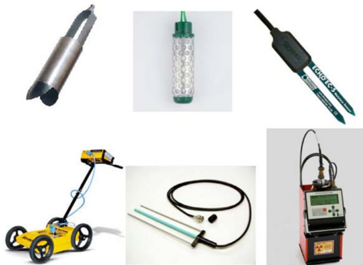
Fig. 3. Soil moisture sensors: Top row: Gravimetric [91], resistive (Watermark) [50], capacitance [17], Bottom Row: GPR [98], TDR [128], neutron probe [92].
