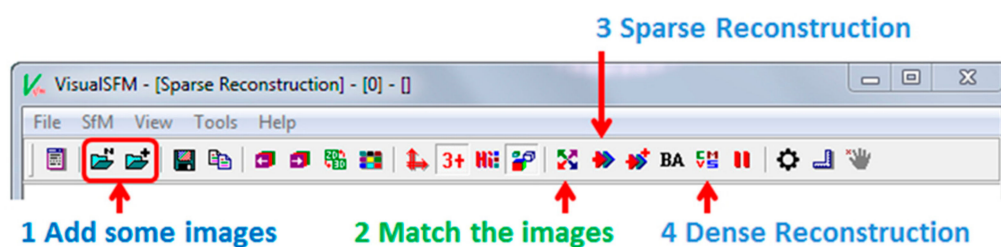
Figure 2. A sample of typical workflow offered by VisualSfM GUI (adopted from http://ccwu.me/vsfm/doc.html ).
