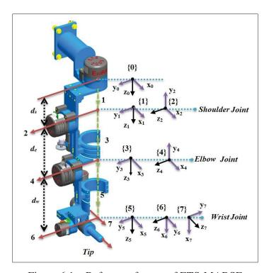
Figure 6.1 Reference frames of ETS-MARSE
