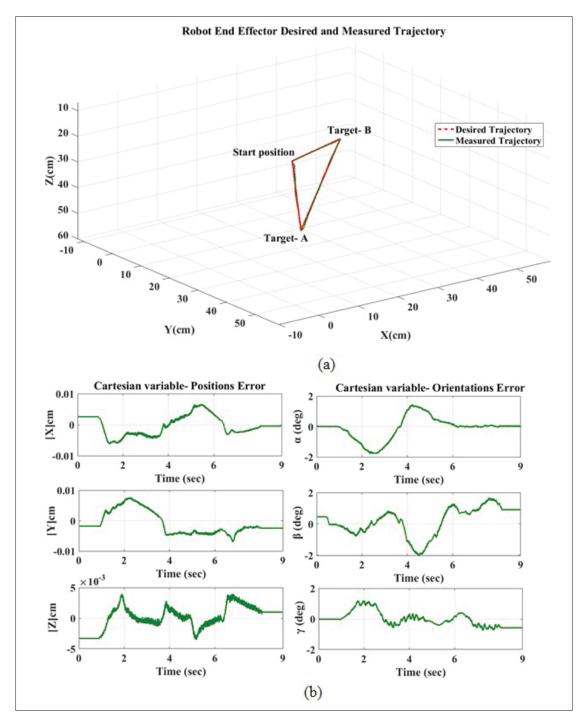
Figure 4.9 (a) Reaching movement exercise, Cartesian trajectory tracking in 3-D space using the conventional controller. (b) Cartesian trajectory tracking error along X-axis, Y-axis, and Z-axis. Experiments was conducted with subject-2 (age: 28 years; height: 173 cm; weight: 72 kg)
