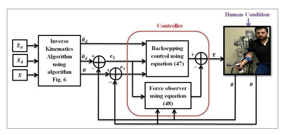
Figure 2.7 General schematic of the proposed control
