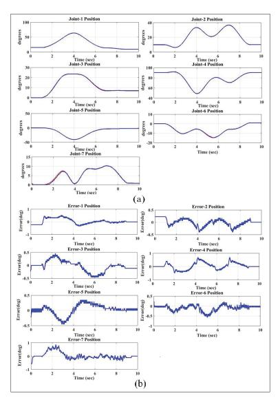
Figure 2.11 Tracking performance of ETS-MARSE in joint space (the inputs of the control joint-based) corresponding to Figure 2.10(a). (b) Tracking error in jointsspace
