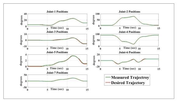
Figure 5.8 Position tracking of the robot in joint space corresponding to the movement performed by Subject-1: (age: 28 years; height: 177 cm; weight: 83 kg)
