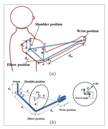
Figure 2.2 (a) Description of human movement in 3D space. (b) Representation of swivel angle  $(\phi)$
