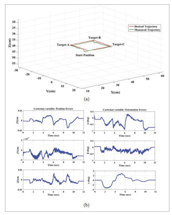
Figure 6.11 (a) Workspace performance of the robot in Cartesian space performed by Subject-1: (age: 27 years; height: 177 cm; weight: 83 kg). (b) Cartesian errors
