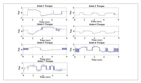
Figure 4.11 Control inputs corresponds to Cartesian tasks using the conventional controller
