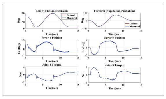
Figure 4.4 General Elbow and forearm motion, trajectory tracking in joint space using the proposed controller. Experiment was conducted with subject-1 (age: 30 years; height: 177 cm; weight: 75 kg)
