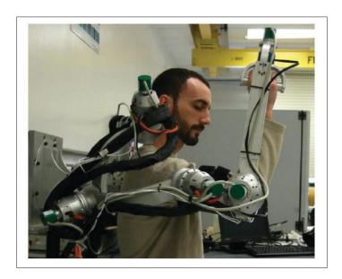
Figure 1.5 MGA Exoskeleton Taken from (Carignan *et al.*, 2007)
