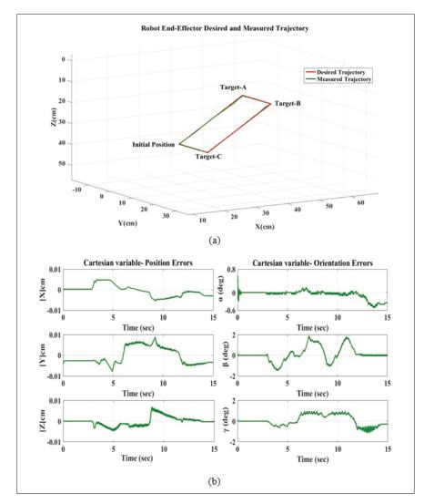
Figure 5.4 (a) Workspace trajectories of the robot in Cartesian space using the proposed controller, performed by Subject-1: (age: 28 years; height: 177 cm; weight: 83 kg). (b) Cartesian errors
