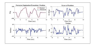
Figure 3.9 Workspace tracking of the robot performed a forearm pronation/supination by subject 1: (age: 29 years; height: 178 cm; weight: 81 kg) using the conventional controller
