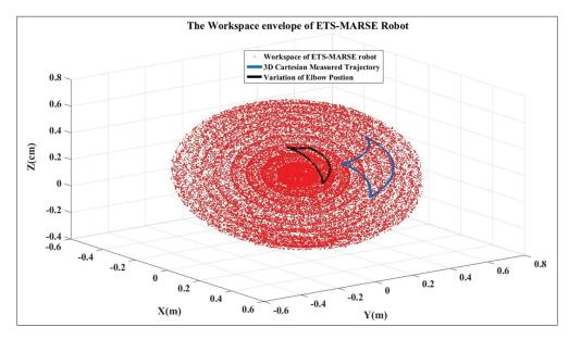
Figure 2.14 Workspace of the ETS-MARSE with performed trajectory corresponding to Fig. 11(a)
