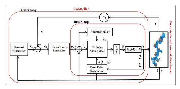
Figure 3.3 Diagram of the compliant control scheme
