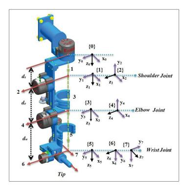
Figure 4.1 Reference frames of ETS-MARSE
