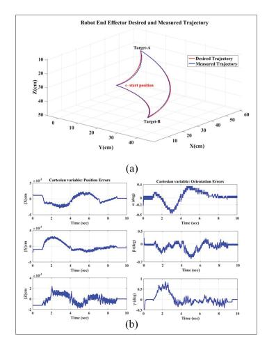
Figure 2.10 Tracking (a) performance of ETS-MARSE in 3-D Cartesian space using proposed inverse kinematics and (b) error in Cartesian co-ordinates (X-Y-Z axes)
