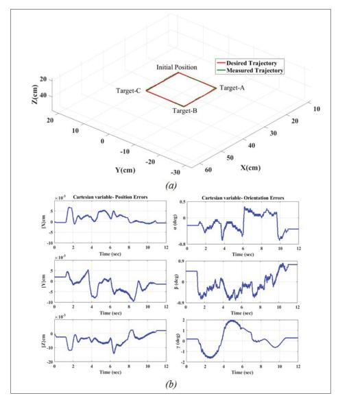
Figure 6.4 (a) Workspace performance of the robot in Cartesian space performed by Subject-1: (age: 27 years; height: 177 cm; weight: 83 kg). (b) Cartesian errors
