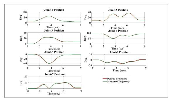
Figure 4.10 Tracking performance of ETS-MARSE in joint space corresponds to Cartesian tasks using the conventional controller
