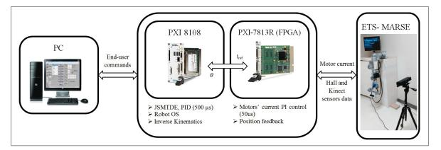
Figure 6.3 Experiments architecture
