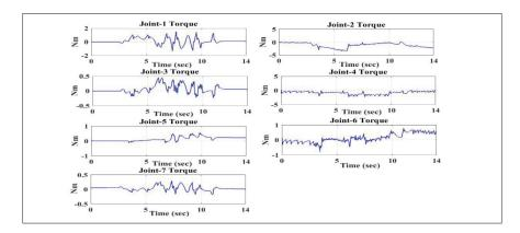
Figure 3.12 Torques input of active rehabilitation task
