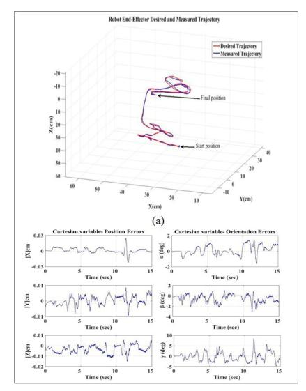
Figure 3.13 Workspace tracking of the robot performed a free motion by subject 3: (age: 27 years; height: 168 cm; weight: 70 kg). (b)
