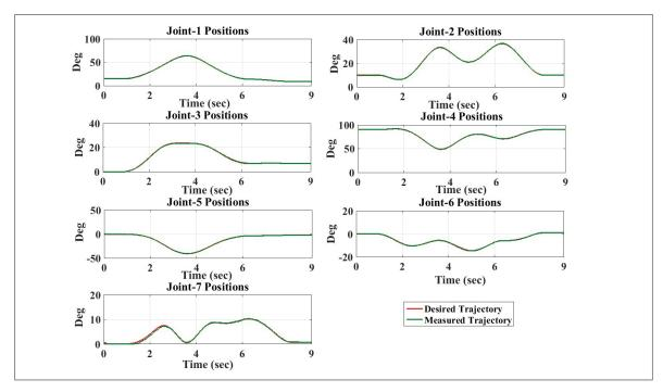
Figure 4.7 Tracking performance of ETS-MARSE in joint space corresponds to Cartesian tasks using the proposed controller
