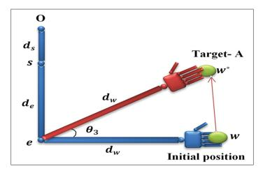
Figure 2.5 Geometrical representation of joint  $\theta_3$
