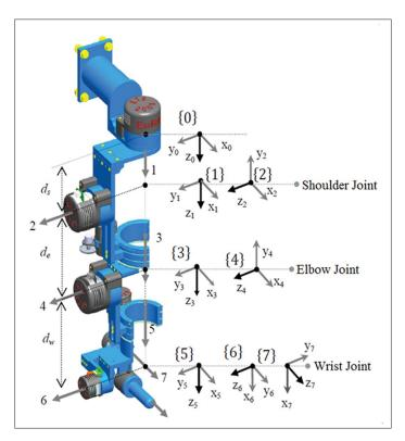
Figure 2.1 ETS-MARSE with link frame
