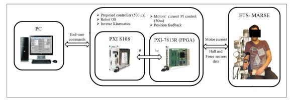
Figure 4.3 General General schematic of experiment architecture (the subject wear the ETS-MARSE robot)
