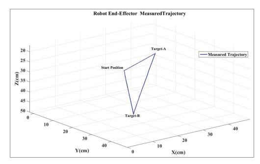
Figure 2.13 Tracking performance of ETS-MARSE in 3-D Cartesian space using proposed inverse kinematics using the B-PIK
