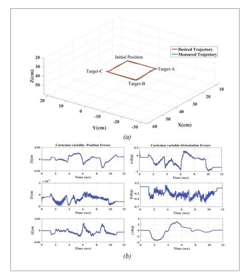
Figure 6.8 (a) Workspace performance of the robot in Cartesian space performed by Subject-1: (age: 27 years; height: 177 cm; weight: 83 kg). (b) Cartesian errors
