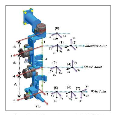
Figure 3.1 Reference frames of ETS-MARSE
