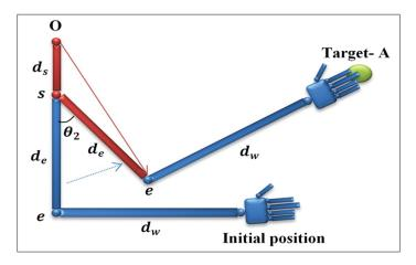
Figure 2.4 Geometrical representation of joint  $\theta_2$
