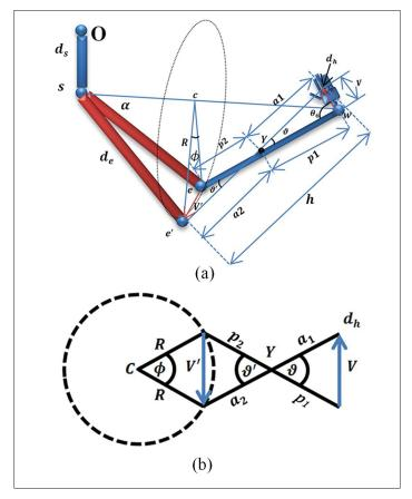
Figure 2.3 (a) Geometrical solution of swivel angle ( $\phi$ ) 3D view. (b) Geometrical solution of swivel angle 2D view
