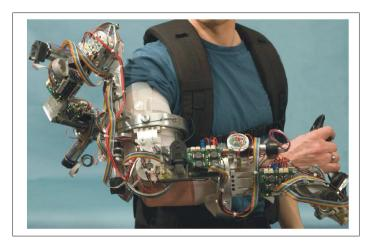
Figure 1.6 SAM Exoskeleton robot Taken from (Letier and Preumont, 2010)
