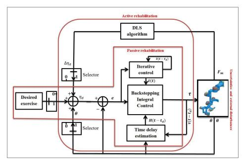
Figure 5.2 General schematic of proposed control (for Selector 1 is pass and 0 is stop)
