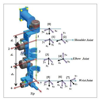
Figure 5.1 Reference frames of ETS-MARSE
