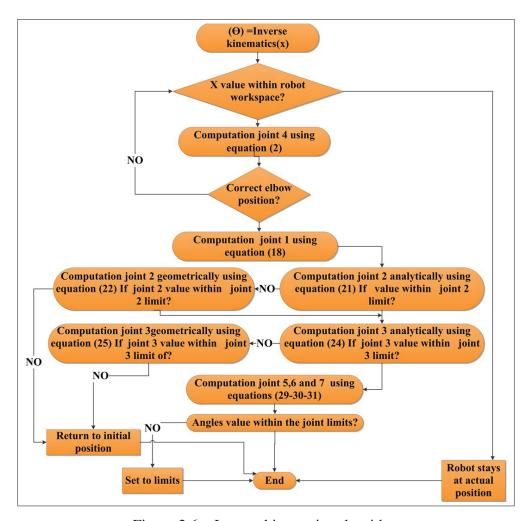
Figure 2.6 Inverse kinematics algorithm
