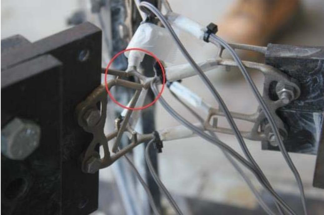
Figure 5-54: One bending node is tested by using the proposed test rig.
