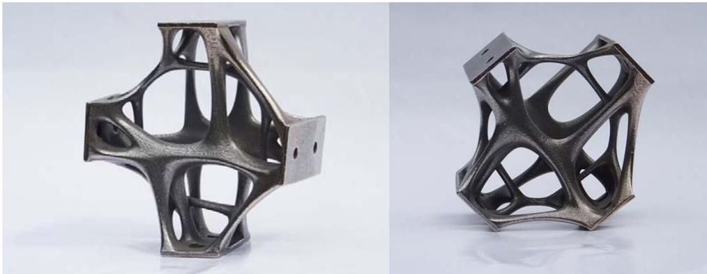
Figure 2-24: Topologically optimised 3D printed node for case study of canopy in Baku International Airport in Azerbaijan [49].
