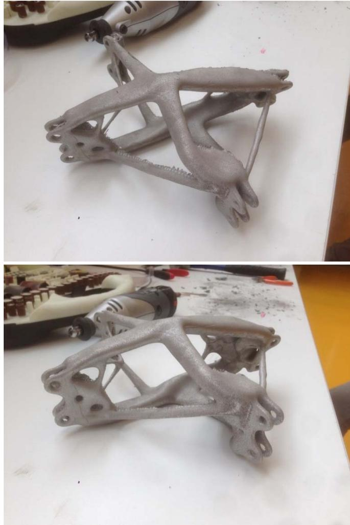
Figure 3-54: Post-processing of a printed metal node.
