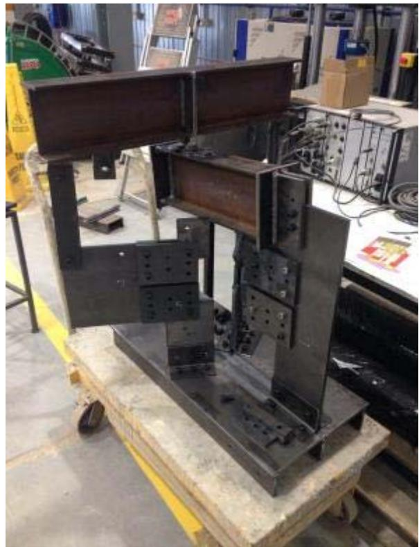
Figure 5-25: The render and picture of the assembled test rig for axial test.
