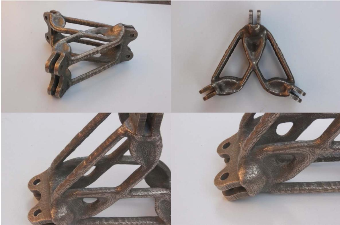
Figure 3-50: In-plane bending node successfully 3D printed by the Binder Jet method.
