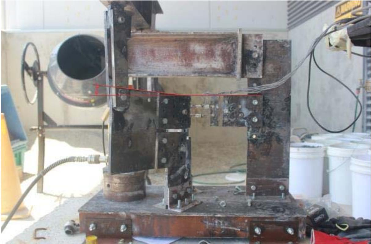
Figure 5-47: The initial rigid rotation in the assembled test setup for axial node.
