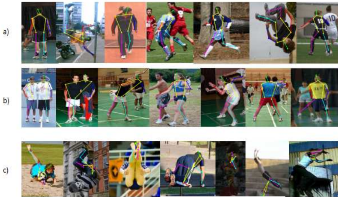
Fig. 4.9 Intuitive estimation results on the LSP dataset. a) Good estimation results. b) Bad estimation results caused by surrounding people. c) Bad estimation results caused by strong pose articulation and low image quality.
