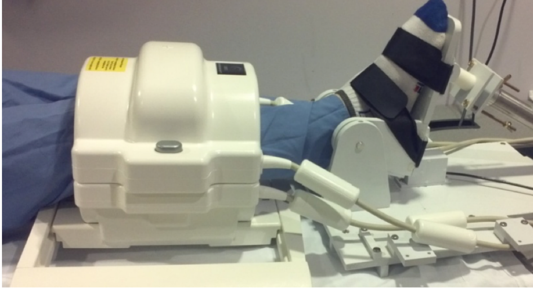
Figure 2.13 Coil positioning around the calf muscle for CrCEST imaging. The right foot was placed into a custom-built foot pedal, operated by a pneumatically controlled piston with constant pressure (set at 7.5 psi for all subjects). A 3-plane, localized image was acquired to determine optimal slice positioning, with the preferred slice containing the largest possible portion of the gastrocnemius muscles (Figure 2.14), determined from the axial image. ( Reprinted with permission (Kogan, Haris et al. 2014). )
