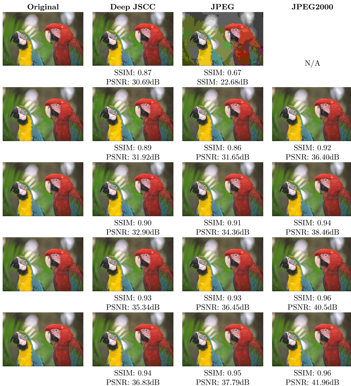
Fig. 11. Examples of reconstructed images produced by the deep JSCC algorithm and the baseline digital schemes that use JPEG/JPEG2000 for image compression for AWGN channel and bandwidth compression k/n = 1/12 . From top to bottom, the rows correspond to SNR values of 1dB, 4dB, 7dB, 13dB and 19dB.
