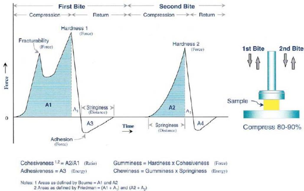
Figure 1. Typical Texture Profile Analysis curve generated by Instron
