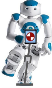
FIGURE 2.7: NAO Robot with the Inverted Pendulum Model [7]
