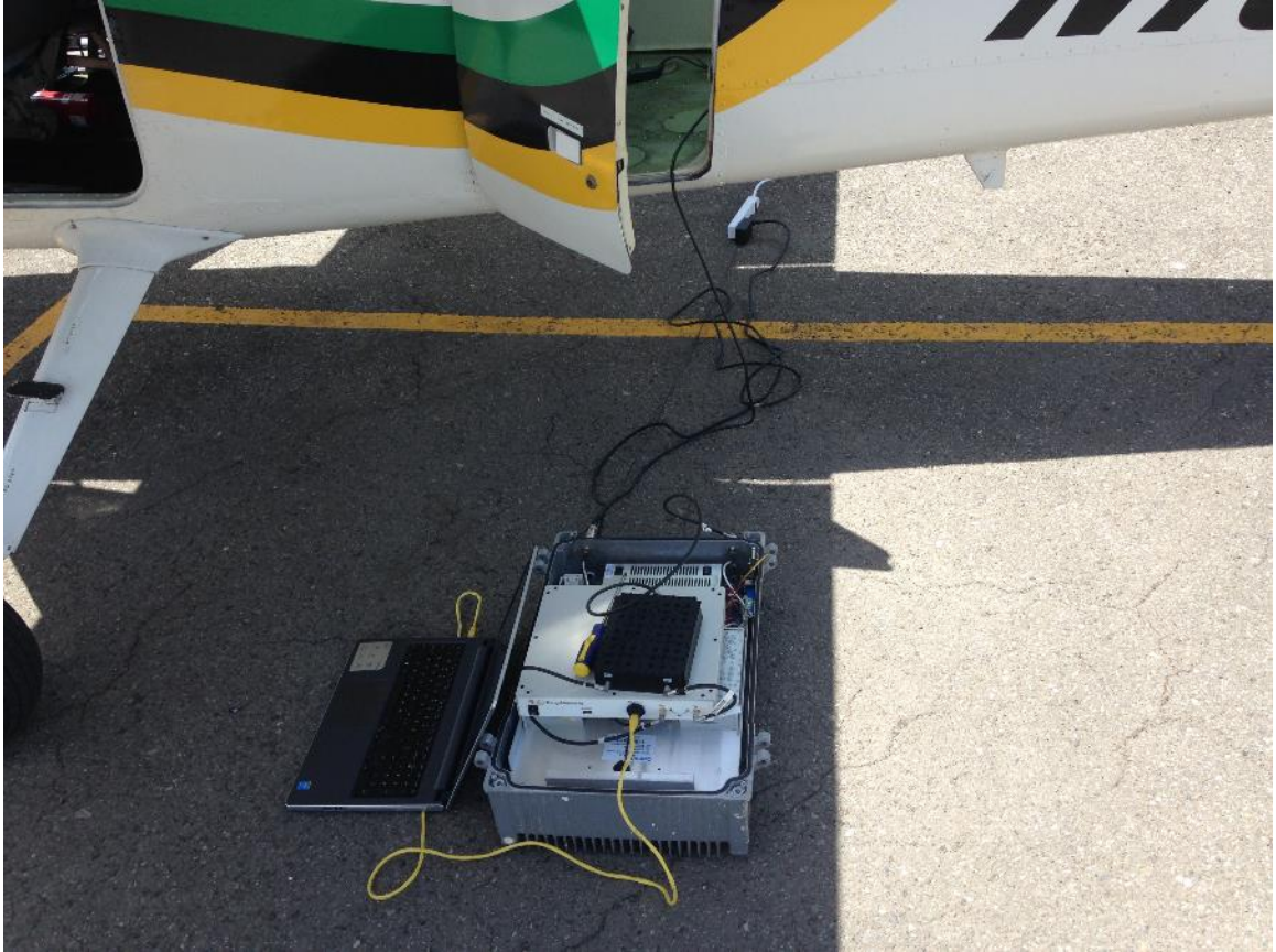
Figure 18. Initial configuration of test network for outdoor environment. The DME antenna is the inverted shark fin on the bottom of the aircraft fuselage in the top right of the photograph.
