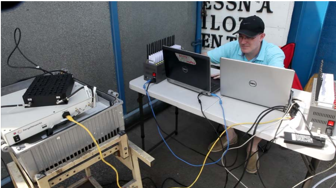
Figure 19. Configuration of test network for outdoor testing prior to installation on aircraft. Shown are the Range Networks network-in-a-box and the two banks of test phones.
