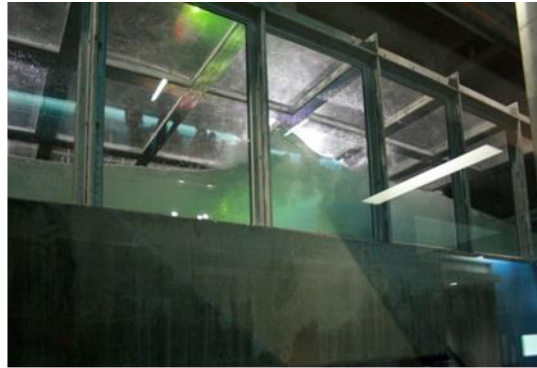
Figure 7. Mechanically generated breaking wave captured from the side of the SUSTAIN tank. Photo Credit: SUSTAIN Laboratory.
