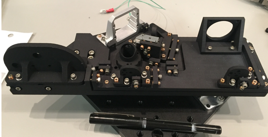
Figure 3-3: The completed assembly of the second iteration of the 3D printed DeMi payload model. All of the components, except for the aluminum DM mount, aluminum FM, and the aluminum feet shown in the image, are 3D printed from Shapeways. The fasteners, bushings and fine adjustment pins are from Thorlabs and are flight-like in order to test hole size and alignment. None of the optics are mounted here, just the optics mounts and the three decks.
