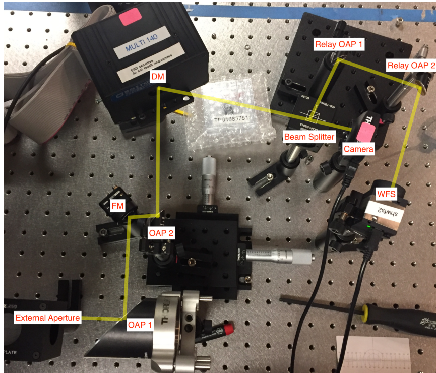
Figure 4-5: Complete bench-top optical system layout of the payload. This setup was produced to perform system testing and individual testing. It was used to verify the WFS operation, the PSF generation on the camera, and for DM actuation testing. This layout is very similar to the final design of the payload optics. We tested several optical layouts before deciding on this one.
