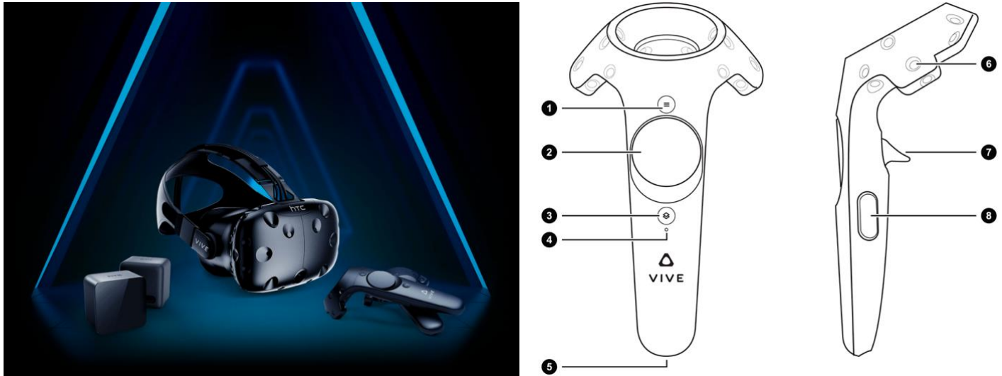
Figure 19 (a, b): (a) Vive VR System, 101 (b) HTV Vive Hand Controllers with Arrows Indicating Buttons and Points for User Input
