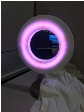
Figure 4. The user's sensor registers a relative drop in BBT. The smart mirror calculates that the user is ovulating, which it indicates with a pink light.
