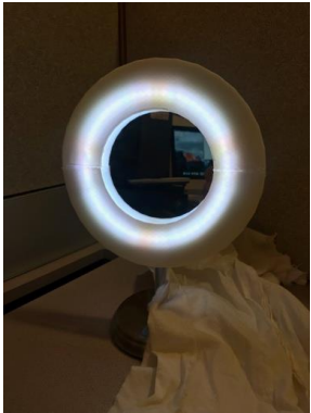
Figure 3. The user's sensor registers a BBT that has dropped from a high; thus the mirror indicates that the user's period is over.
