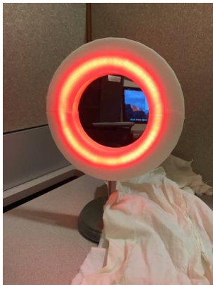
Figure 2. The user's sensor registers an elevated BBT, and the smart mirror calculates that they are on their period, causing the LED lights to shine red.
