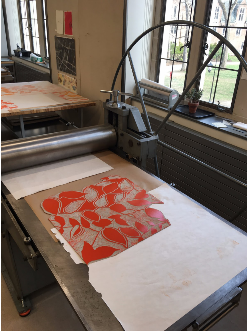
Figure 18: Relief printing process: inked linoleum block on the French Tool Press.
