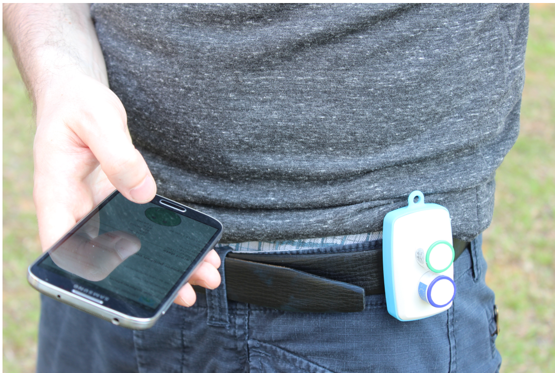
FIGURE 2.3: Participants were given portable sensors (shown right) that transmitted pollutant concentrations and descriptive air statistics via bluetooth to their cellphones every 20 seconds.
