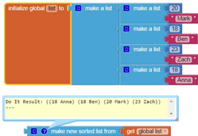
Figure A-11: Given a list of lists, the basic sort operator sorts by the first index of each sublist.
