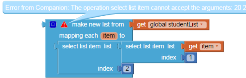
Figure 5-7: Returns an error because it is not possible to use two select list item blocks on item, which is a list, not a list of lists
