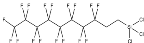
Figure 1-10: Chemical structure of heptadecafluoro-1,1,2,2-tetrahydrodecyl trichlorosilane.
