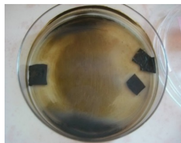
Figure 3-8. Oxidized dopamine solution and dip-coated polymer substrate, indicated by the dark brown color.
