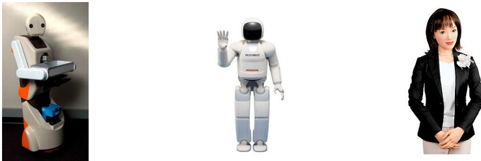
Figure 7.5. The mechanical social robot, Snackbot (left), the humanoid social robot, Asimo (center), and the android social robot, Actroid DER (right)
