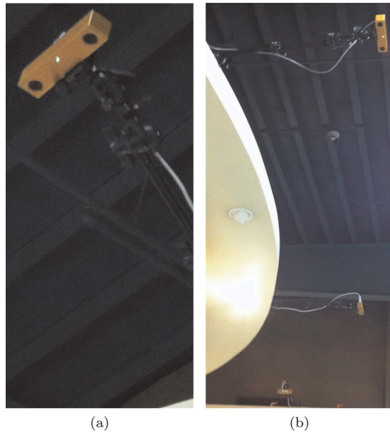
Fig. 14. (a) Stereo camera used by our pedestrian tracker and (b) three stereo cameras, configured to maximize coverage and track quality.
