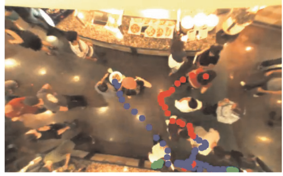
Fig. 6. An example trajectory of a cafeteria patron. The trajectory was hand labeled and segmented; blue dots are part of the nominal trajectory (modeled with the kernel function k = k_{linear} + k_{matern} + k_{noise} , as in Section 3.1.3), green dots are goals, and red represents interaction between agents (see Section 3).
