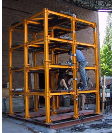
FIGURE 1: STEEL-FRAME SCALED BENCHMARK STRUCTURE.
