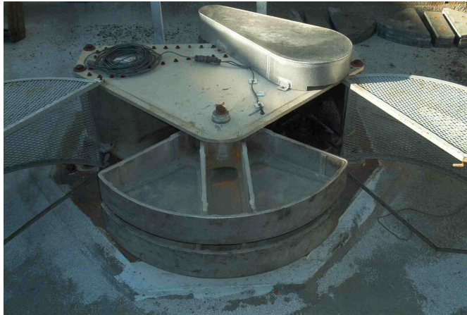
Figure 4. Kinometrics VG-1 Synchronized Vibration Generator (Shaker). The counter-rotating buckets, shown empty, can be loaded with different configurations of lead weights. The shaker is located on the roof of Millikan Library, as shown in Figure 2.
