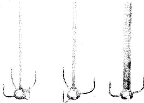
Fig. 9. View of total load samplers for 33.5-inch flume. (Flow is downward at sampling point.)
