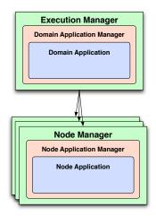
Figure III.1: OMG D&C Architectural Overview and Separation of Concerns
