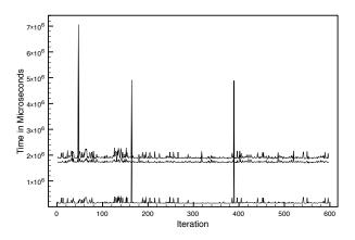
Figure IV.5: Latency Jitter for 1000 Component Deployment
