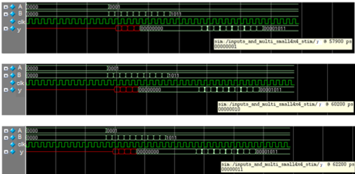
Figure 33: Golden serial-implemented full adder multiplier with outputs
