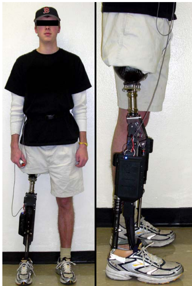
Figure 2-11. Unilateral transfemoral amputee test subject used for the powered prosthesis evaluation.
