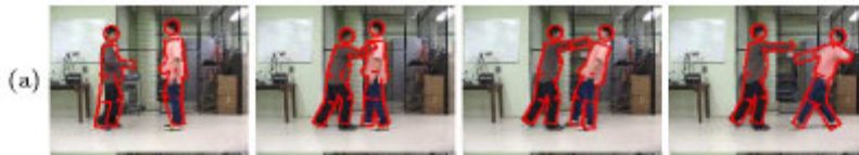
Figure 3: A sequence of tracked model states indicating a push [25]
