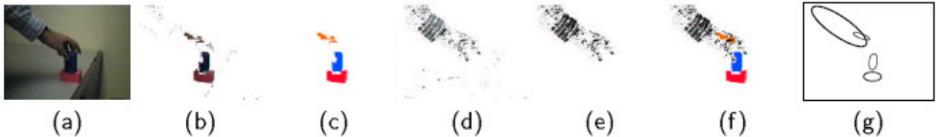
Figure 21: The processing stages of Siskind and Morris's tracker. (a) shows an input image. (b) shows the coloured pixels. (c) shows the output of the region grower on (b). (d) shows the moving pixels. (e) shows the output of the region grower on (d). (f) shows the combination of (c) and (e). (g) shows the ellipses that are fit to regions from (f) [68]
