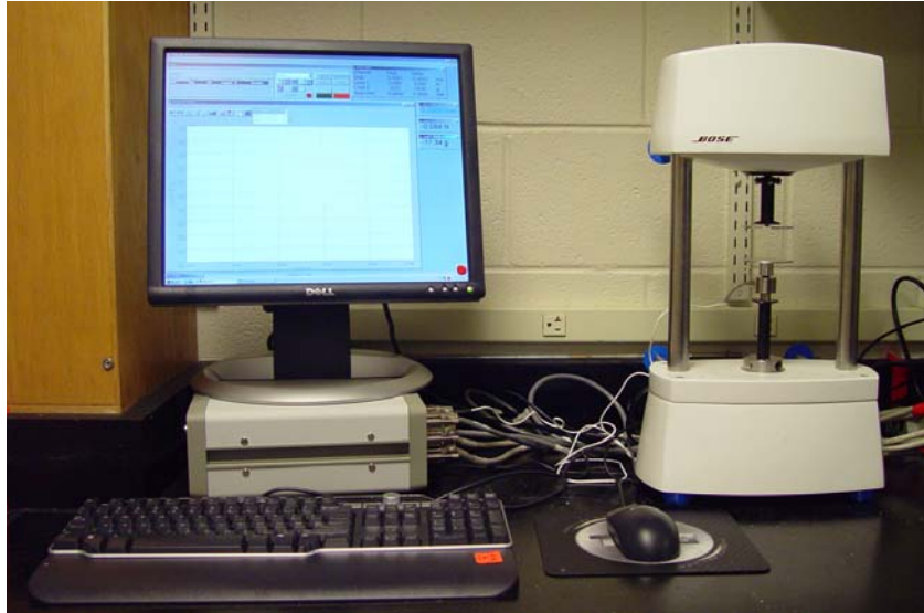
Figure 2. Material testing setup used for gel and liver testing.
