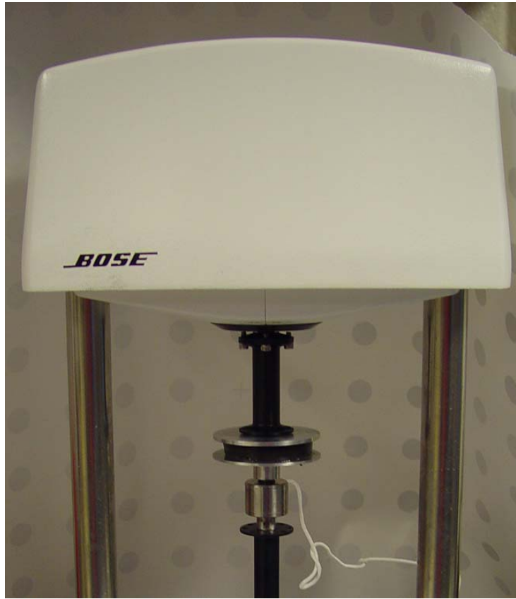
Figure 4. Gel compression testing setup.
